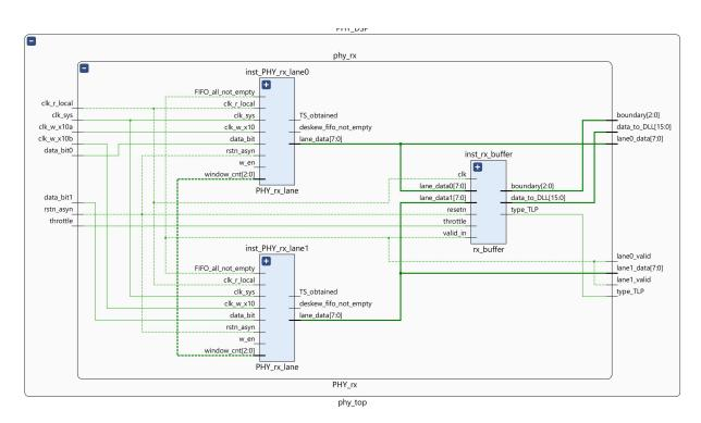
Rx\_PHY Data Deserializer: Un-striping buffer used to group 2-byte data (1 byte from each lane) to DLL.
