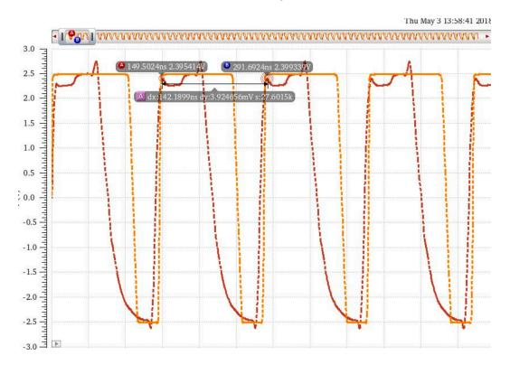
As the graph shows above, the clock has a period of about 142 ns, and since I will only use the clock to trigger the counter, the positive edge of the clock is the only thing that matters in this case.
