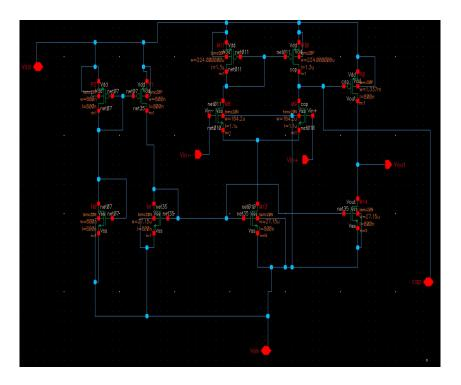
Some of the transistors were 1000 times larger than the others, which is not optimal. I tried to decrease transistor sizes as much as possible, connecting the larger transistors was very tedious.
