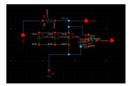
The capacitor was split purposely into three instead of using 50pF which could be quite large for one single capacitor.
