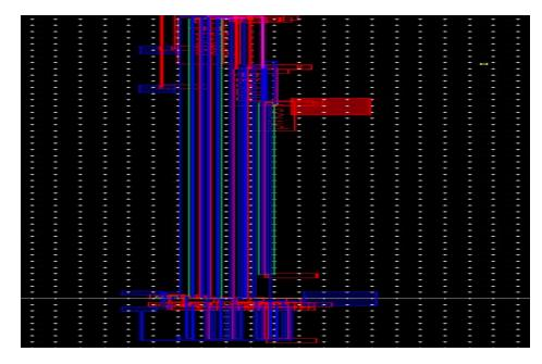
I tested my Op-Amp by sweeping the positive input terminal and grounding the negative one - the output switched from rail to rail at a difference of 50  $\mu$ V which was good enough for my purpose.
