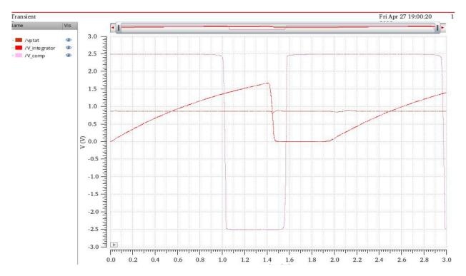
As you can see, when the integrator and Vptat voltage intersect, there is a slight time delay and then the comparator switched to LOW. After a delay of about 0.5 µs (which is about 5 clock cycles) the integrator's capacitor is discharged and the whole process repeats again. It is worth noting that the comparator switched to HIGH slightly earlier than the capacitor starts recharging which can induce some error on additional runs after the first one.
