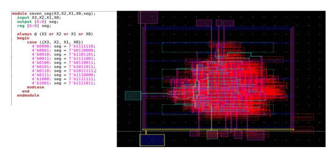
Seg<6> will be connected to pin A, Seg<5> will be connected to pin B, and so on.
