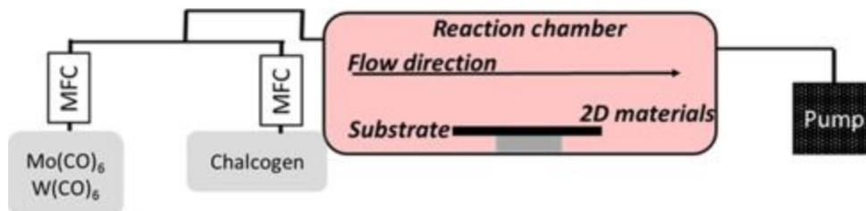
Figure 10. The schematic of an MOCVD reactor for TMD synthesis. (Adopted from Ref. [10]).
