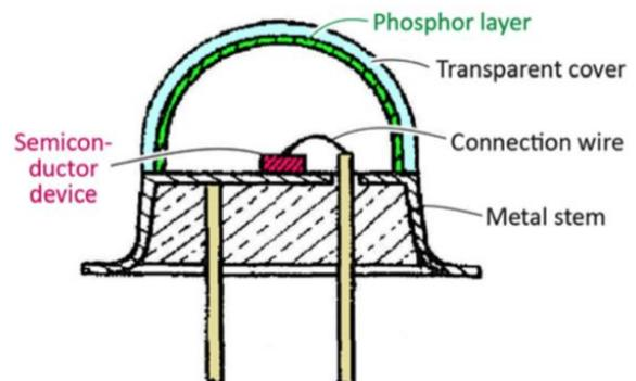
**Figure 6.** LED structure having an LED chip exciting a phosphor that is coated on the inside of transparent cover. The arrangement of the phosphor is reminiscent of a fluorescent lamp that has the inside of a glass tube coated with a phosphor (adopted from Ref. [6]).
