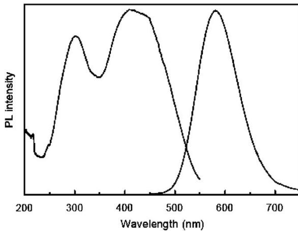
Figure 7. Excitation and emission spectra of  $\text{Ca}_{0.925}\text{Eu}_{0.075}\text{Si}_9\text{Al}_3\text{ON}_{15}$ . The excitation and monitoring wavelengths are 420 and 581 nm, respectively. (Adopted from Ref. [8]).
