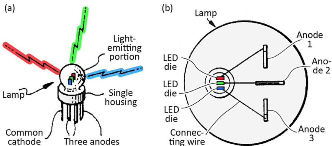
**Figure 5.** (a) Perspective view and (b) top view of multi-LED-chip white LED consisting of a red (R), green (G), and blue (B) LED chip (or die). Optical mixing of the RGB emission components results in white light (adapted from Ref. [6]).
