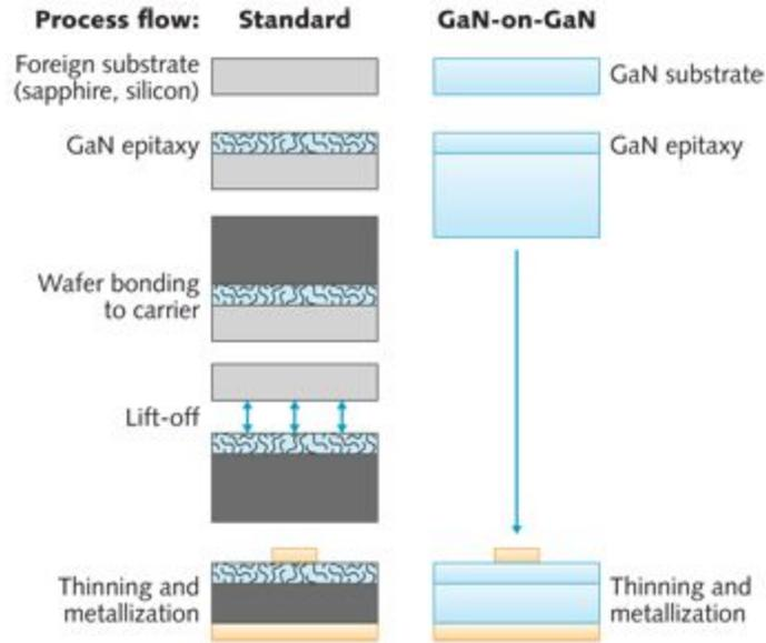
Figure 9. A semiconductor manufacturing flow chart for LEDs. (Adopted from Ref. [9]).
