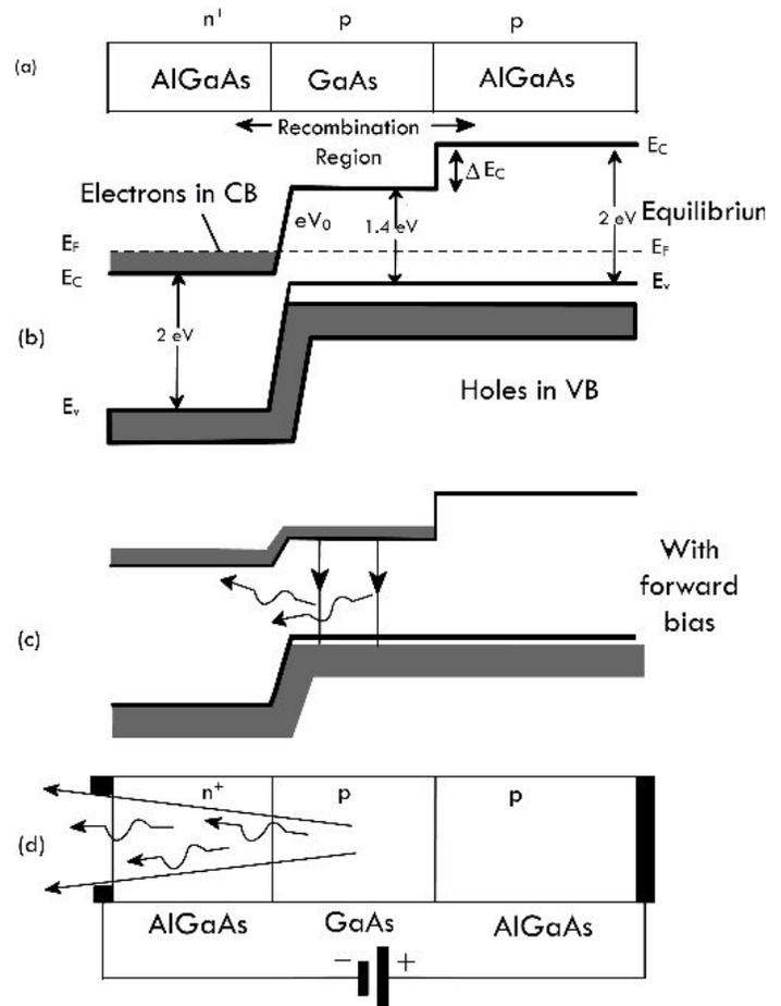
Figure 3. Double heterostructure based LED. (a) Device structure. (b) Equilibrium band diagram. (c) In forward bias electrons and holes are injected in GaAs. (d) Visible light emission.
