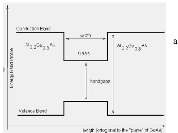
Figure 1. Sketch of Semiconductor Heterostructure of Quantum Well Type. (Adopted from Ref. [2]).
