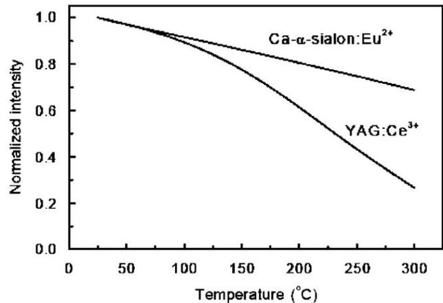
Figure 8. Temperature dependence of emission intensities of Ca-a-sialon:Eu<sup>2+</sup> and YAG:Ce<sup>3+</sup>. (Adopted from Ref. [8]).
